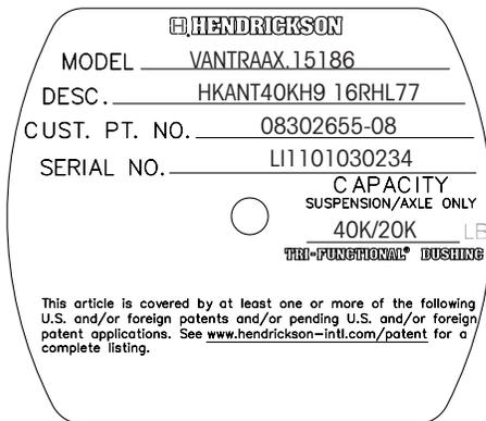
**Suspension ID tag**, for sliders, located roadside front, on slider rail above frame bracket or on frame bracket. For HT and INTRAAX, located inward side of curbside suspension beam.
