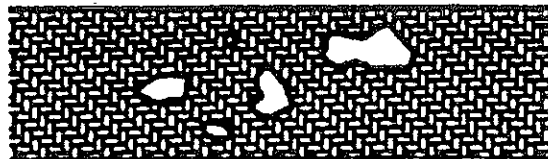
Figure 5 Melting Or Charring Of The Tie Down, Or Weld Spatter On The Tie Down
