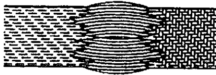
Figure 3 Excessive Abrasive Wear
